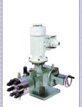
Performs excellent especially in accurate feeding into ultra-high pressure processes. This exquisite hydraulically driven metal diaphragm pump is typically featured in precision feeding of low flow into very high pressure thanks to its mechanical durability with no allowance for process liquid permeation through the diaphragm into the hydraulic chamber.
